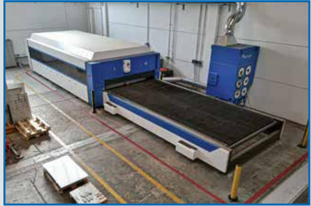
TAGLIO LASER TECNOLOGIA FIBRA FINO A SP. 20 MM FIBER LASER CUTTING UP TO THK. 20 MM
